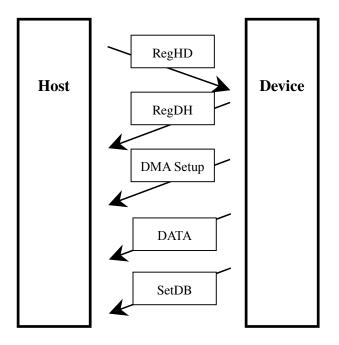
Figure 5.18 READ FP DMA QUEUED command protocol
